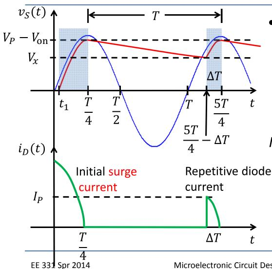
Charge lost due to discharging replenished by charging current during  $\Delta T$ :
