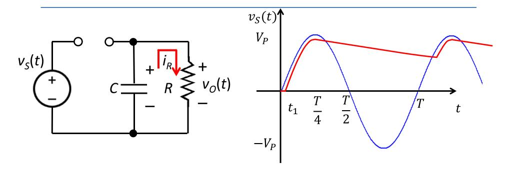
After t = T/4, diode OFF, capacitor discharge via R,  $v_O(t)$  slowly decreases (exponentially), until in the next period,  $v_S(t)$  becomes larger than  $v_O(t)+V_{on}$  again
